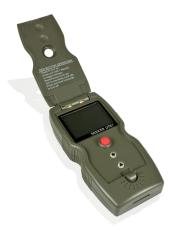
Seeker Lite<sup>2</sup> analyzes the detected RF energy and automatically rejects all noise and signals that are not caused by leaks from your system.
